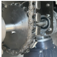
Automatic chain lubrication
