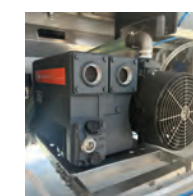
Vacuum pump inside machine frame
