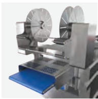
Rewind system with motorized rolls
